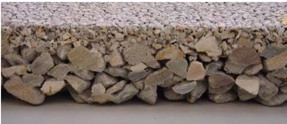
Rys. 9. Struktura nawierzchni dwuwarstwowej (Evaluation of U.S. and European Concrete Pavement Noise Reduction Methods, National Concrete Pavement Technology Center, 2006)
